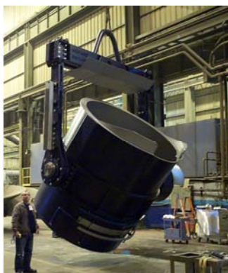
ACETARC-50T CAPACITY WORKHORSE LADLE WITH MOTOR GEAR ROTATION AND INVERTER SPEED CONTROL AT ROLLS ROYCE NAVAL MARINE (USA)
