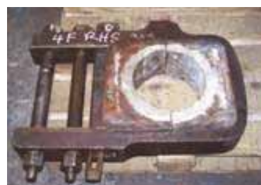
Re-Engineering of Con Rod Big Ends white metal coated and machined to original tolerances.
