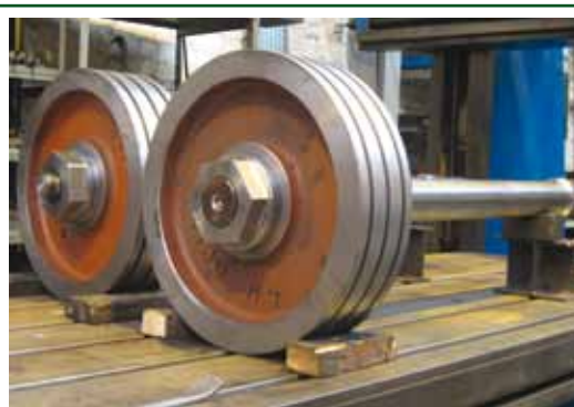
Brand new Pistons and Re-Engineered Piston Rods for Locomotive BIG JIM
