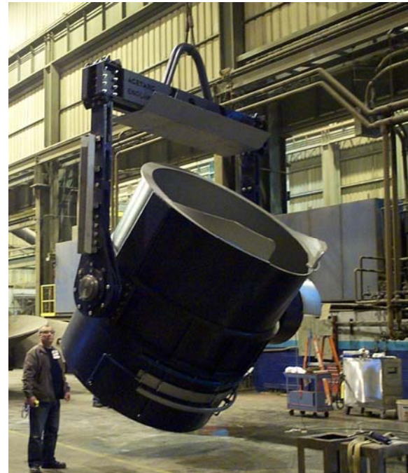
50t Acetarc motorised ladle undergoing commissioning at Rolls Royce Naval Marine Pascagoula Foundry USA
