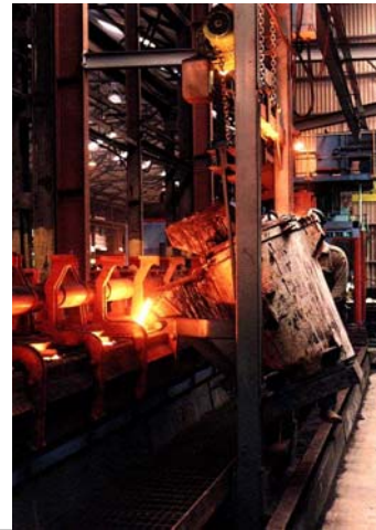
50t Acetarc motorised ladle undergoing commissioning at Rolls Royce Naval Marine Pascagoula Foundry USA
